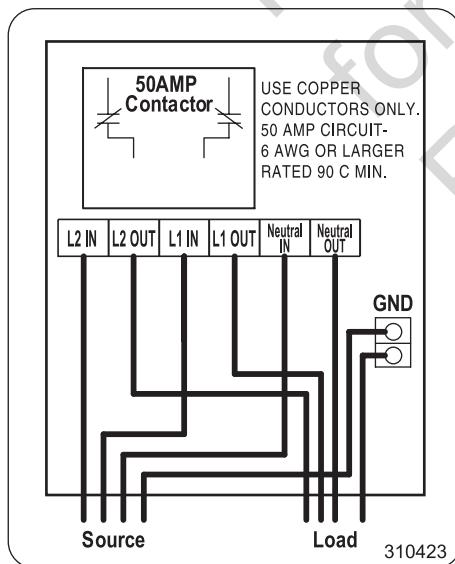
6. For a 240VAC appliance/load, locate the line conductors between the main distribution panel and the managed appliance/load. Terminate the line conductors in the remote module to "L1 IN" and "L2 IN" terminals (E).
