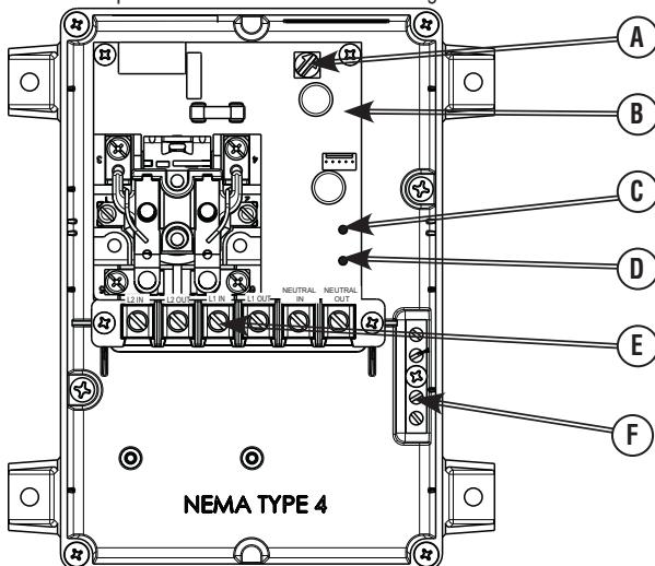
7. Locate the neutral conductor between the main distribution panel and the managed appliance/load. Terminate the neutral conductor in the remote module "NEUTRAL IN" terminal (E).
